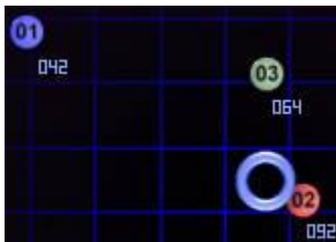
In this picture, the intensity of the sound will be at 92 % on the speaker 02, 64 % on the 03, and 42 % on the 01, and the perception must be the visual position of the blue Ring. However, this may be different according to the place from which you listen to, the acoustic characteristics of the room and, don't forget, the nature of the sound !
