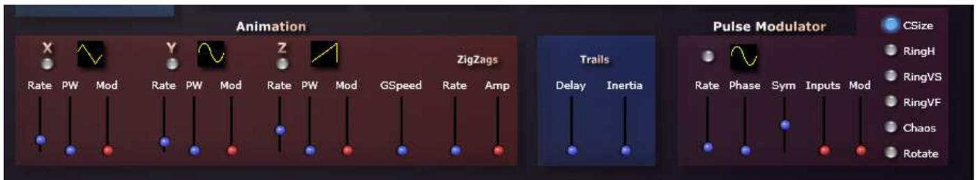
The first three control groups activate and determine the values of three LFOs (waveform, speed, square wave ratio and amplitude), each modulating the position of input # 1 (and only this one) according to the three axes of space. The other seven inputs just follow the movement (see below).
